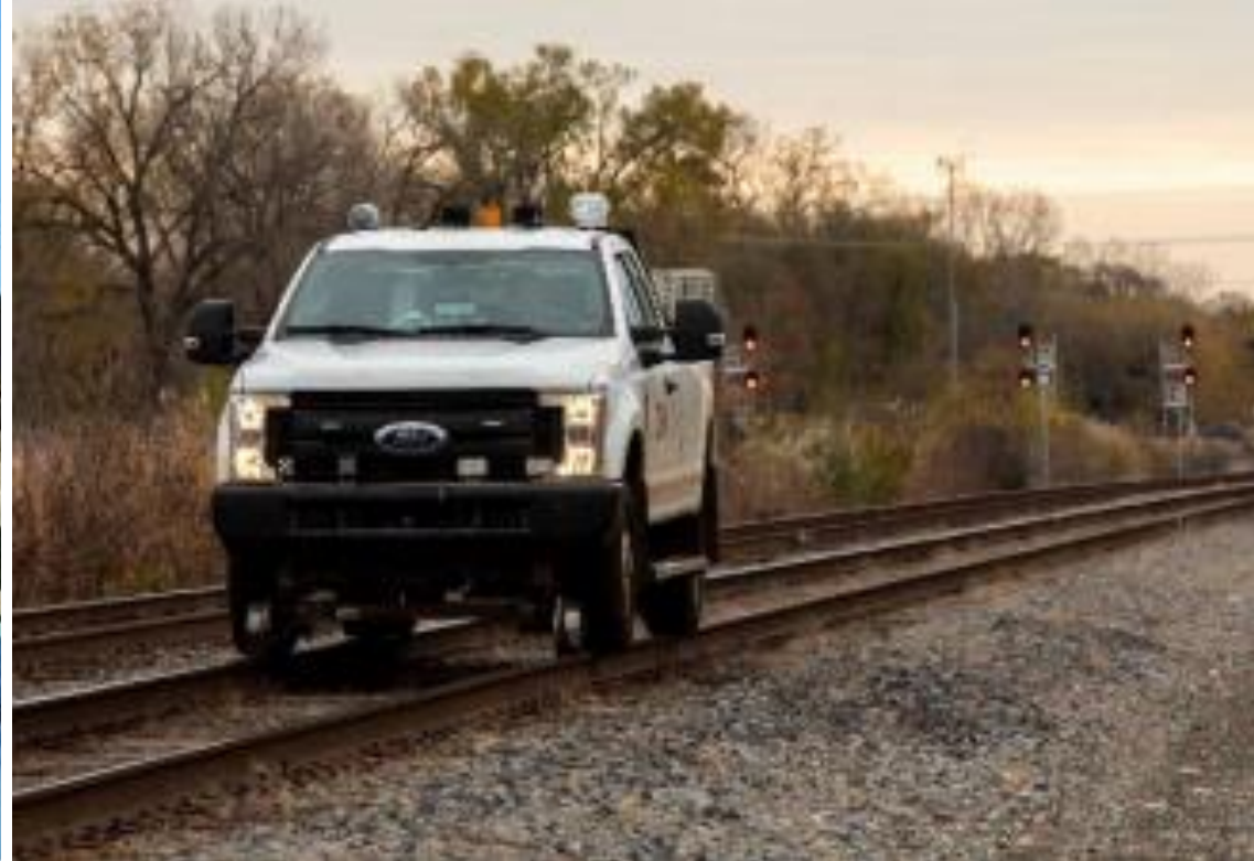
CN Hi-rail in the field: Revenue trains cannot occupy the same track while the hi-rail is performing a visual inspection
